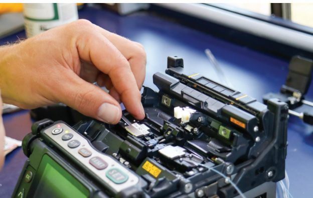
Pictured: Splicing fiber during our fiber builds.
